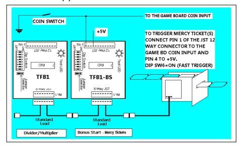
The mercy ticket input is an opto isolated input. In this example it is assumed that the coin switch operates 5V logic input of the game board, therefore the Pin 4 of the JST 12 connector is connected to +5V.
