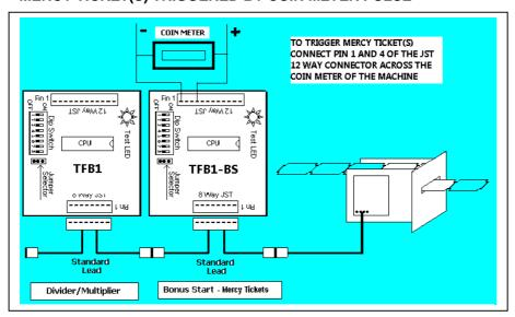
The opto isolated mercy ticket input can be connected directly across the 12V coin meter. This input can handle 5 to 30V DC. Note that the positive side of the meter is connected to the Pin 4. If the Dip Sw 6 = OFF (delayed trigger) fast successive pulses will be ignored, tickets will be triggered by the last pulse only.
