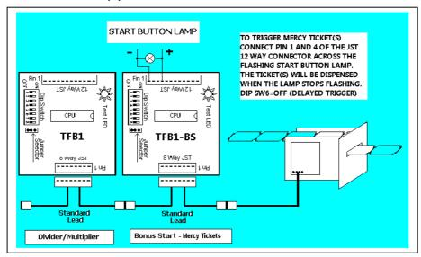
In this example the mercy ticket input is connected across a start button lamp, which starts flashing when the machine is credited. When the game starts and the lamp stops flashing, this event triggers the mercy ticket(s). The Dip Sw 6 = OFF (delayed trigger).
